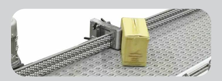
Suitable for use in dry or washdown environments, this ARB<sup>™</sup> Case Turner provides consistent, repeatable package positioning at discharge.
