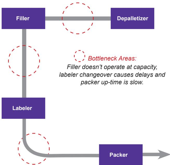
Layout A illustrates four machines in a production line, each operating at 90% efficiency. Whether planned or unplanned, the machines in this example almost never shut down at the same time, resulting in a loss of 40% efficiency.
