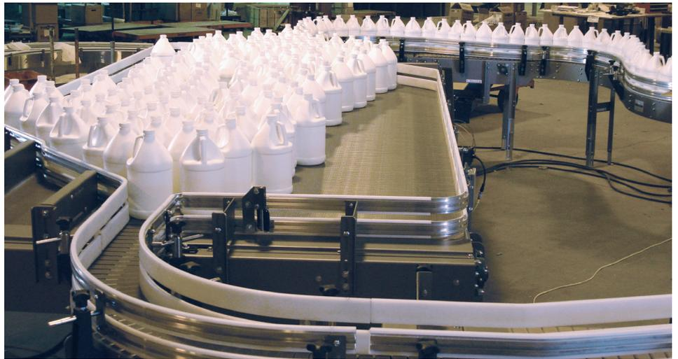
*Re-Flow Accumulation Table showing In-Line Accumulation*
