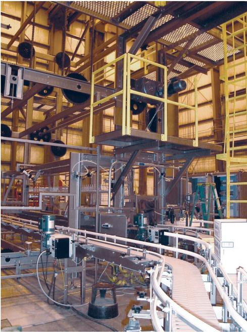
*This is the in-feed / drive side of the Rolco FILO (First-In, Last-Out) Accumulator, also showing bypass conveyors.*
