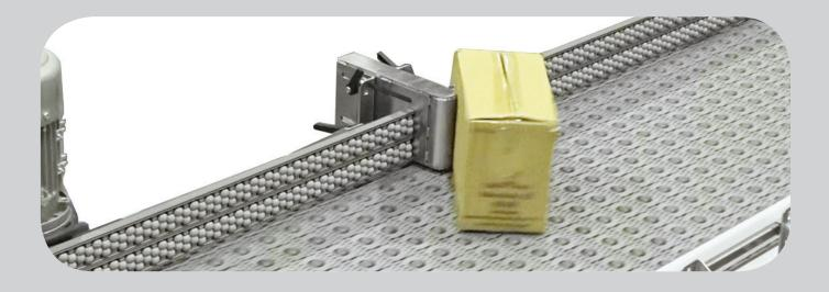
Suitable for use in dry or washdown environments, this ARB™ Case Turner provides consistent, repeatable package positioning at discharge.
