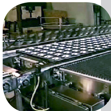
Highlighting both a wire mesh belt conveyor and a dual strand belt conveyor, multiple pans are transferred at 90 degrees.
