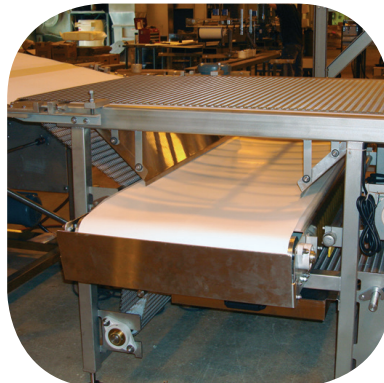
This reclaiming system uses a trough belt positioning under a wire mesh product conveyor to capture and reuse salt.
