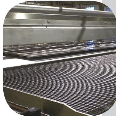
Shown is a 12 ft. wide wire mesh conveyor and a servo sweep device pushes eight pans at a time.
