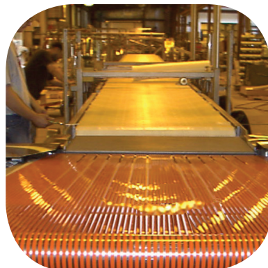
This urethane belt system spreads products after being cut in upstream operations.
