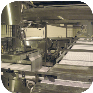
This is a servo controlled indexer designed for effective right angle transfer and metering of the baking trays.
