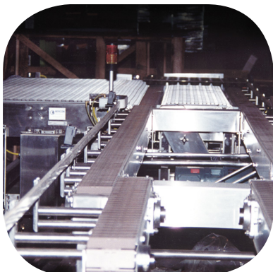
This dual strand pan system features an upstream 90 degree pop-up transfer and an overlap transfer in the foreground, providing smooth and effective pan conveying..
