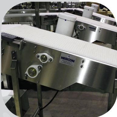
Nercon manufactures oven terminal ends in various widths and drum diameters. Drive ends include motors, reducers. Idle ends include pneumatic take-up assemblies
